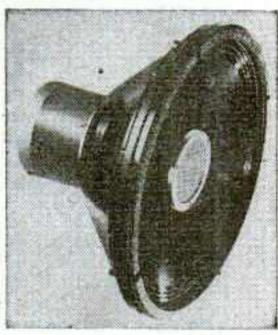
The following are the manufacturer's specifications and performance claims; nominal response is 30 to 15,000 cps, power rating is 30 watts (U. S.), impedance at 400 cps is 15 ohms, bass resonance is 40-45 cps and crossover frequency is 2,000 cps. The speaker is available in the U. S. thru Ercona Corporation, N. Y. C.
