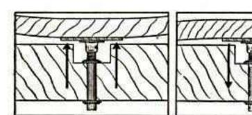
Using ordinary screw-driver, turn right to PUSH up a "valley" in table . . . turn left to PULL down a "hill" to insure smooth surface that attracts repeat-play. 4 separate Stabilizers may be adjusted in any combination of PUSH and PULL, guarding all 4 quarters of table against play-killing. profit-eating warpage.
