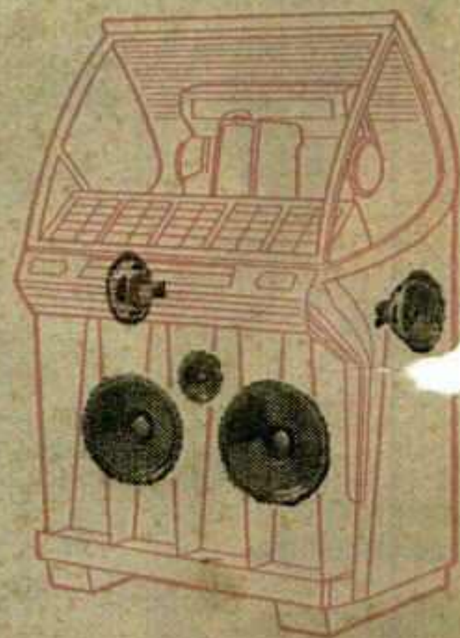
Mounted at the front of the acoustical chamber are two heavy-duty, 12-inch low-frequency speakers and a 5-inch high-frequency speaker. Wide-range 8-inch speakers are mounted on either side.
