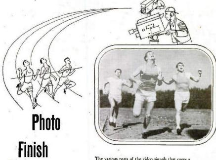
The various parts of the video signals that carry a television picture through a coaxial cable travel at different speeds. When they leave the studio, they accurately represent the scene before the camera. But, like sprinters, some are faster than others and pull ahead in the "race" to the receiving point.
