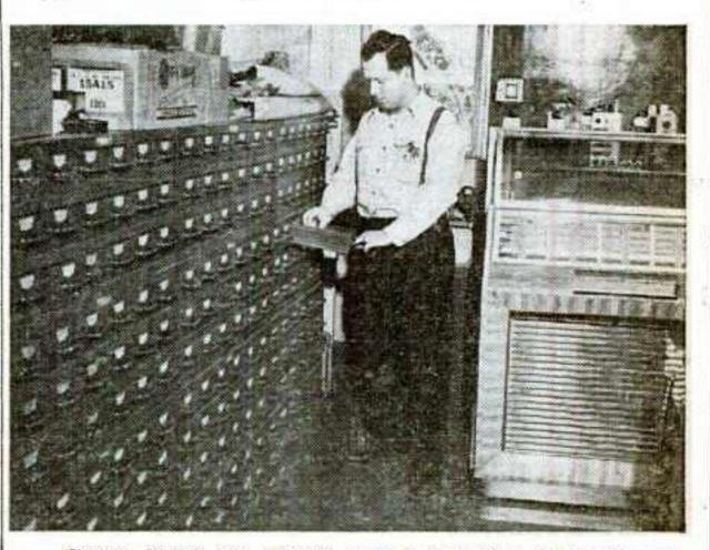
SMALL PARTS BIN OFFERS convenient stocking of miscellaneous nits vital to continuous trouble-free operation. Individual drawers, numbered and carrying labels describing contents, permit easy checks on spare parts backlog plus enabling operator to find given items in the least possible
