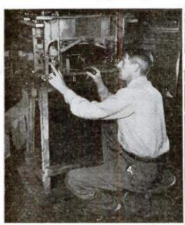
PREVENTIVE MAINTENANCE pays off for one Chicago operator, Frank Padula, who has devised a special rest block for mounting changer mechanisms for a thoro parts wear and functional check. Changers brought in for any and all defects are gone over completely, offen resulting in prevention of future play interruptions by removing parts not yet giving trouble but showing signs of doing so.
