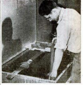
ANOTHER ASPECT of preventive maintenance is cleanliness. Using a cleansing solution and a good-size tank or tub as a degreaser such as is used in industrial plants, the operator can dunk both small and large juke parts equally well. An easy brush-off after removal from the solution usually serves to whisk away undesired accumulations of drift and grease. Here a Seeburg record assembly is being cleansed of foreign matter which could affect disk delivery.
