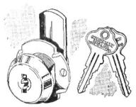
No. 4750 Improved Herculock-pick - resisting design, "Shark-tooth" keyway, Double sided key. Wrench-proof cylinder, Extra heavy spur washer, retaining screws, and key. Cam movement 90 degrees. Thousands of key changes. \*Trademark registered
