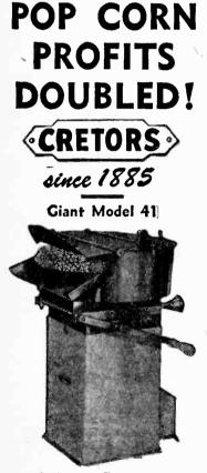
Large production . . . Fast. efficient, trouble-free. Pops corn direct in the seasoning and salt. Pan easily dumped. . . Enclosed transmission . . gears run in oil. . . . Keeps heat where needed. . . No pressure from popping corn insures maximum popping volume. Dump handle interchangeable ... right or left hand operation. Machines operated by bottle gas or natural gas. Motor driven by electricity. Gasoline extra. Pops 50 lbs, corn per hour.
