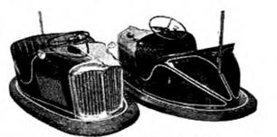
1935 AUTO-SKOOTER CAR T HE Auto-Skooter is designed with streamlined body, richly decorated, chromium - plated radiator shell, front wheel drive with transmission enclosed, free wheeling, cushioned axles, steel faced bumper, electrically lighted cowl lamps, deep cushioned upholstery, soft rubber steering wheel.
