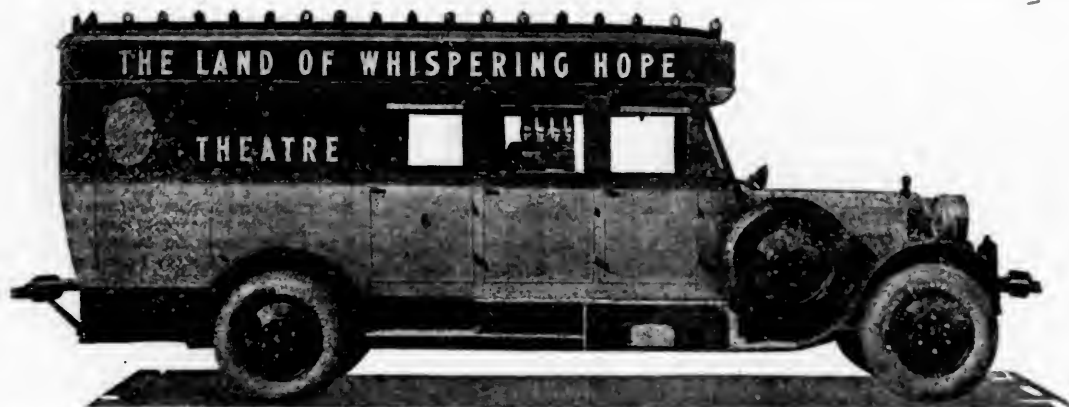
Burr Nickle, of Los Angeles, has one of the finest and most elaborate air calliope outfits in the world (illustration above) used for publicity work in his big production, "The Land of Whispering Hope". Built at a cost of nearly $30,000, it is on a specially constructed Reo speed chassis with 18-inch wheel base, has a Tangley self-playing calliope, which uses standard rewind piano music rolls, and also has a keyboard so that it can be hand-played, the same as a hand-played instrument. The car has balloon tires, and the inside is arranged like the interior of a Pullman car. It has berths, toilet, washstand and practically every convenience of a hotel except a bath. It has a compartment for the musical instrument, another for the feature films, and living accommodations and berths for the manager and assistants. The entire outfit is 18 feet long. It is Mr. Nickle's plan to go into a city, book the film, advertise it and play the date, thus cutting out the usual distribution thru film agencies.
