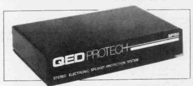
QED Audio Products' Protech SP150 is a handy companion to loudspeaker drive units — it protects them from overloading. Deriving its power from the signal source, the SP150 constantly monitors the signal to the speakers. In the event of an overload, a time delay is triggered. If the level doesn't drop to within a lower range, a relay cuts the power to a safe measurement.
