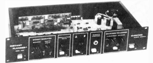
**Eventide Clockworks Inc.** has introduced a plug-in card for their "Instant Flanger" unit, which gives the unit "Instant Phaser" capability. This plug-in card, the BPC101, is interchangable with the SDC-1 Flanger Card and utilizes electronic phase-shift networks to generate frequency cancellations in the audio signal, rather than the bucket brigade devices used in the Instant Flanger.
