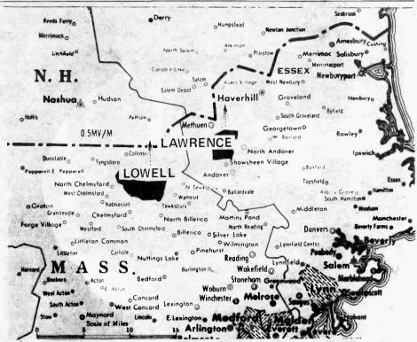
TALE OF TWO CITIES — This coverage map shows the two cities Lowell and Lawrence from which WLLH transmits its dual signal. Each city has a tower and transmitter of its own with the signal coverage of the twin transmission set-up shown in the white area.
