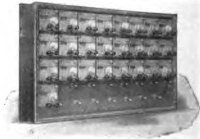
AUTOMATIC CALLING DEVICE FOR TRAIN DISPATCHERS' OFFICE. (Cover Removed.)
