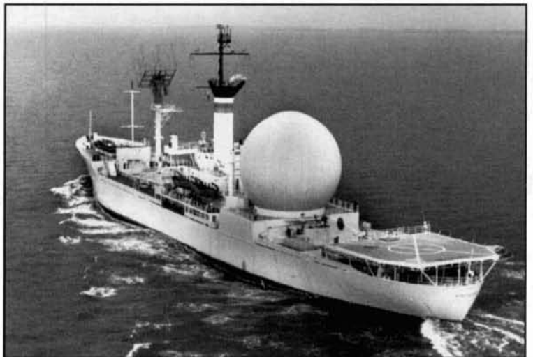
Photo J. Aft view of the USNS Kingsport AG-164. Notice the satellite disk radome behind the ship's house and stack.
