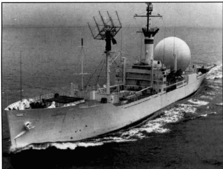
Photo K. Forward view of the USNS Kingsport AG-164. Notice the two high-frequency discone cages on the forward decks. Directly behind is another satellite tracking antenna, composed of helical antenna array mounted on one post forward of the ship's house. Aft, on the ship's house, are more 35-foot whip antennas for high-frequency communications.
