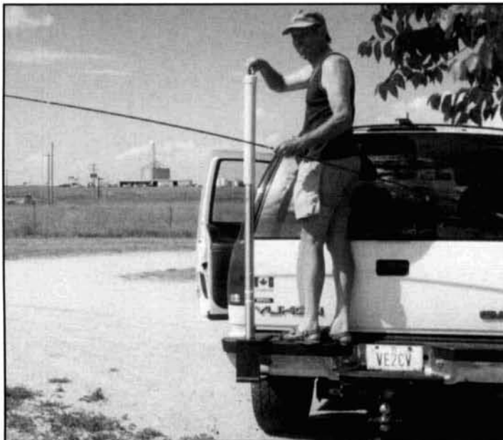
Photo B. VE2CV installing the full-length 4.9-meter whip.
