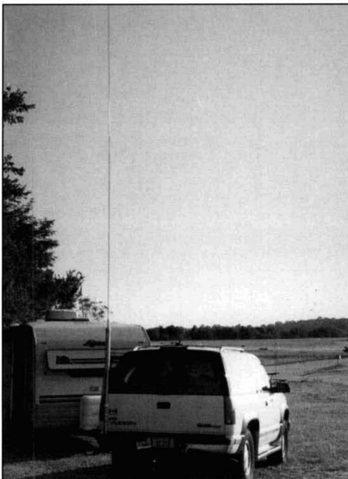
Photo C. The full-length 4.9-meter whip on the truck.
