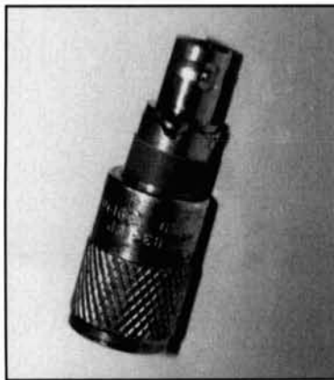
Photo A. The author's PL-259 to female BNC adapter.
