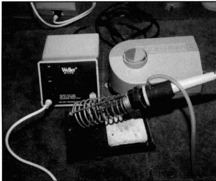
Photo B. The Weller soldering-station power supply, modified iron, and aquarium air pump used in the author's home SMD soldering setup.
