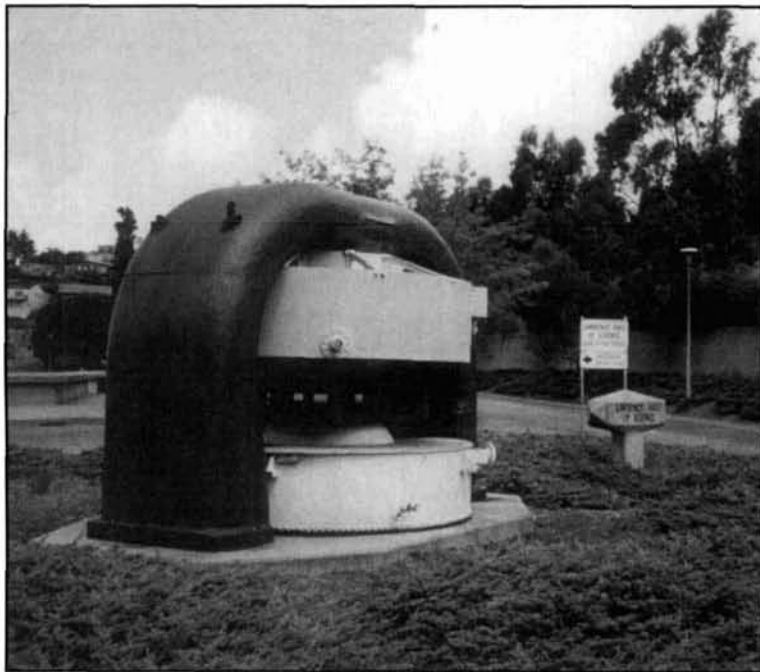
Photo B. A large steel casting for a megawatt-sized arc transmitter donated to Berkeley and Lawrence by Fuller.
