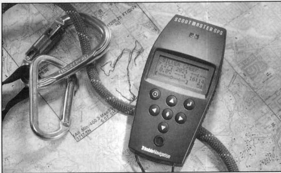
Photo A. The Trimble Scout GPS™ handheld unit has the Maidenhead Grid Locator System built into its software. The unit's RS-232I/O port lets you upload and download location data to and from your computer.
