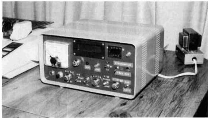
Photo A. The super-slow receiver. Two separate decoder/displays are used. At the upper center of the panel is a 32-character LCD. To the right is a four-character LED display. The two decoder-displays operate in parallel. The meter monitors AGC voltage and outputs of the various phase detectors, as well as crystal-heater and battery voltages. This particular receiver can be set to four different channels (out of 3000 possible).
