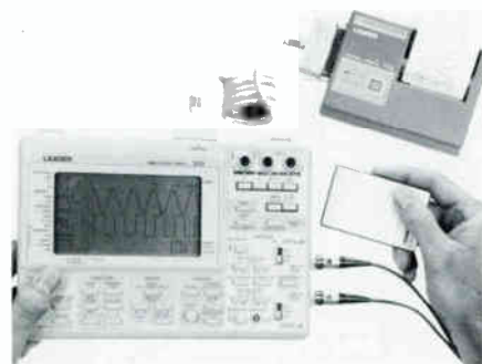
The Model 300 portable 30-MS/s digital storage oscilloscope from Leader.
