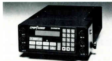
Christie's CASP/2000 universal programmable battery support system.
