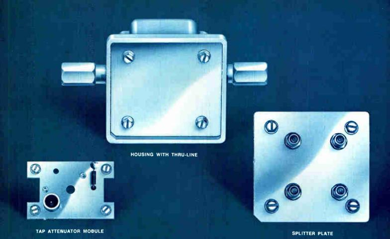
We designed the model 1400 as an economical directional tap (housing with thru-line, tap attenuator module, splitter plate) to enable installation of the housing only during construction and later adding the tap attenuator and splitter plate ... without interrupting service.
