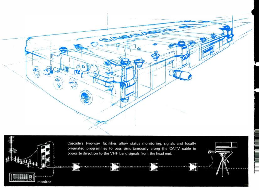
The output level of individual trunk amplifiers may be monitored constantly, day and night, at the head end or at any control point along a trunk line.
