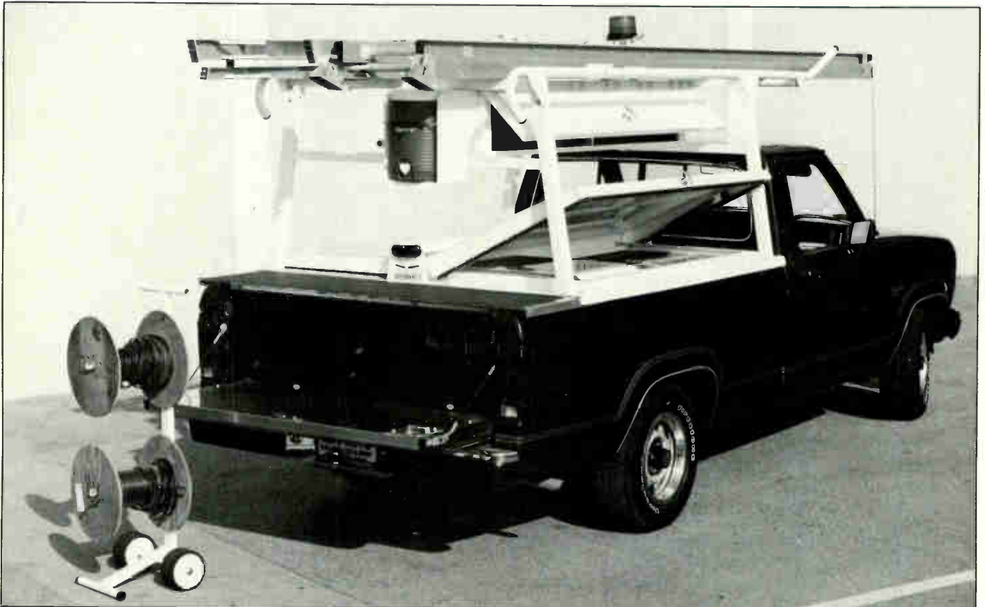
Tailgater TruckBed System, outfitted as an installer truck, showing the work deck, upper cabinet, ladder lock and beacon bracket, water jug, rolling parts tray and cable caddie.
