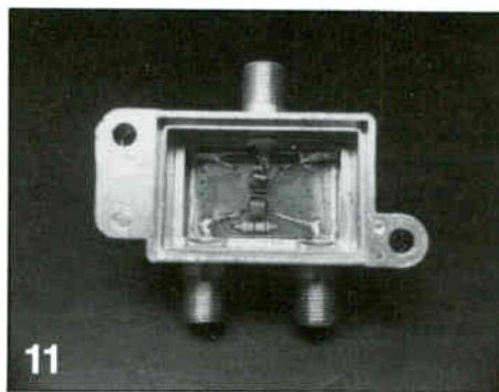
11 A higher quality printed circuit board two-way splitter.
