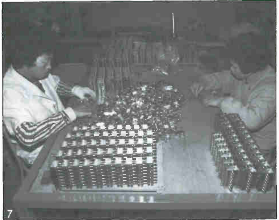
Assembly line workers install inserts into the cases.
