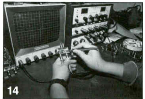
14 Finally, the splitters are tested and aligned.
