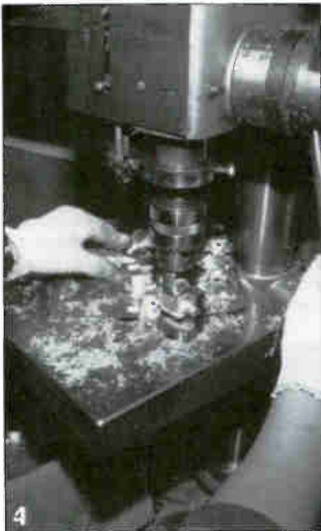
Each part of a splitter or tap needs to be threaded so the proper connector can screw on.
