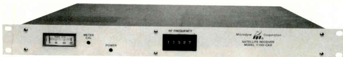
1100 CKR C and Ku Band 950-1450 MHz Compatible with LNB's
