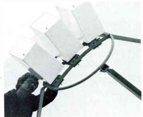
When installed on a 5-meter antenna, isolation between beams is better than 20 dB, with a loss of about 1 dB at 4° off boresight.
