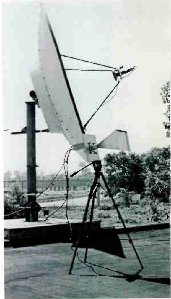
Microwave interference phase canceller attached to a TVRO system. The standard gain feed horn (with LNA) is pointed directly at the microwave interference.
