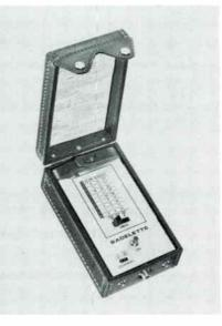
Bar Graph dB read-out, allowing the installer to operate the meter in the carrying case.
