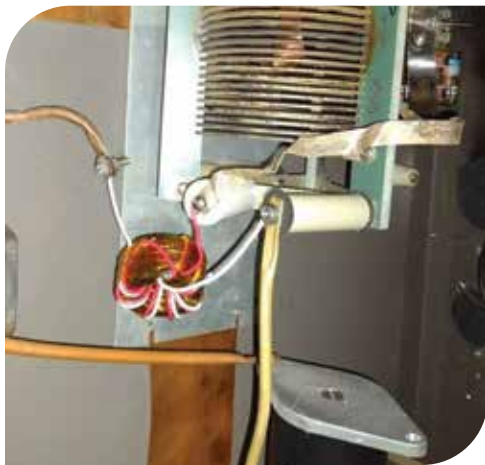
Figure 2. Prototype 1:4 UnUn 2.4" diameter type 77 ferrite core
