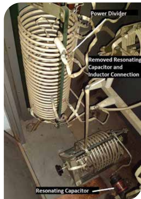
Figure 3. WION phasor power divider; resonating network removed
