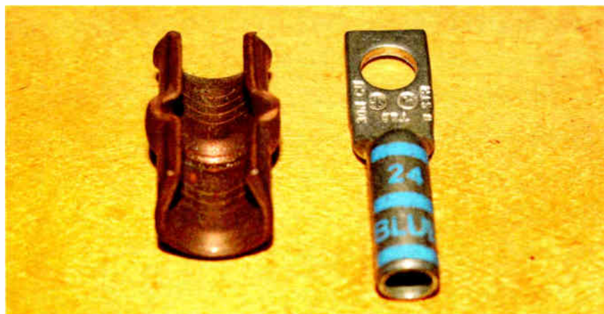
Fig. 2: You can crimp connections to the down conductor using a C-Tap and lug.
