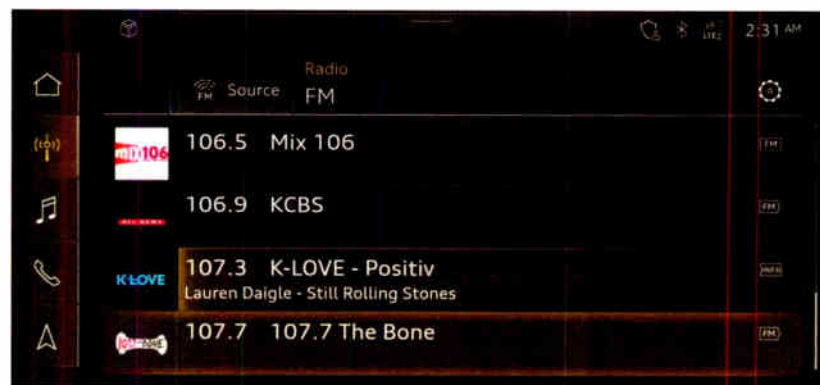
How a hybrid radio display looks in an Audi vehicle. A small box at right indicates whether the active station source is "FM" or "Web."
