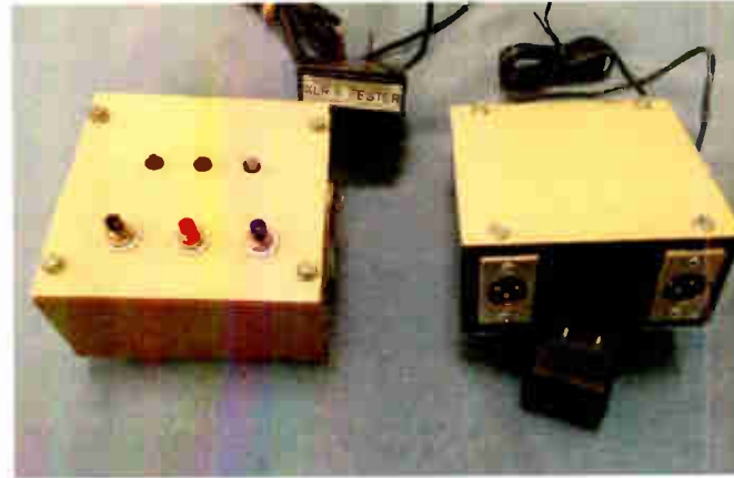
Fig. 4: No, your eyes aren't playing tricks. When you build the Buc Fitch project that we told you about last month, the box should have male and female XLRs. (The box on the right is a balanced-to-unbalanced converter.)
