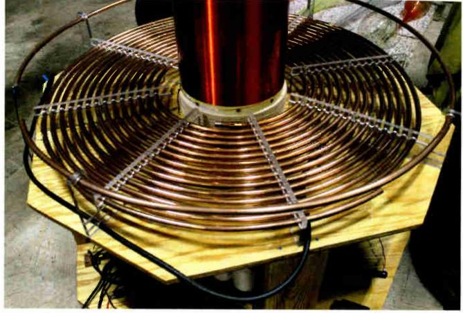
This "pancake" inductor wound with copper tubing forms the primary of the Tesla coil. The heavy black wire connects to an adjustable "tap" that allows tuning of the primary circuit. The elevated copper ring is used to protect components (including the IGBTs) mounted under the base.
