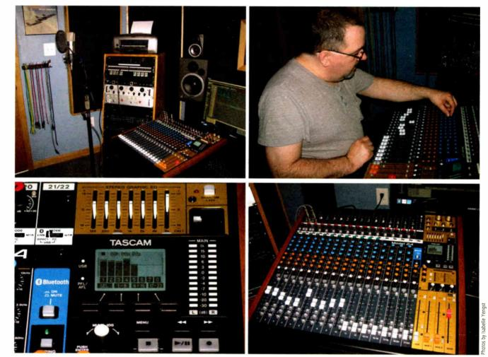
output section features faders for stereo output and monitor busses, as well as a fader for a separate submix. There are separate controls for control room monitors, headphones, and solo. There is a built-in FX section featuring a few basic reverb and delay settings, along with master aux controls. The output section also includes a basic seven-band graphic equalizer that can be assigned to the main stereo bus or the monitors. A global phantom power switch is provided for the mic channels.
