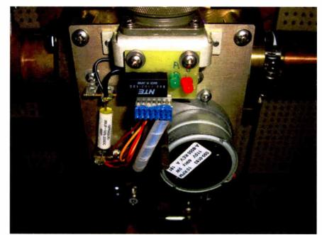
Fig. 3: The latching relay board remounted with the diagnosing LEDs in place.
