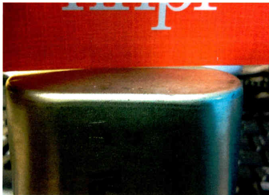
Fig. 1: Hold a business card along the top of this failed capacitor and you can see the slight bowing, indicating failure.
