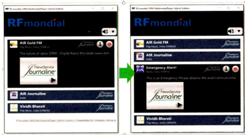
Audio programs on one frequency in a normal situation and with the insertion of an emergency alert with normal programs temporarily suppressed
