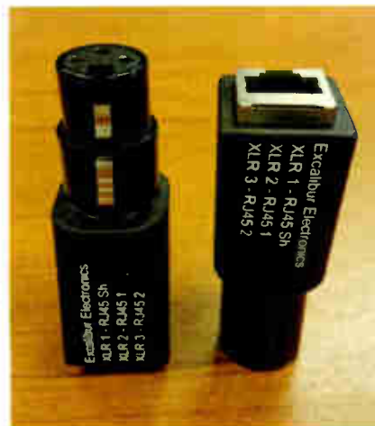
Fig. 6: The female version — note the silk-screened pinout on the adaptor.
