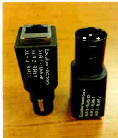
Fig. 5: The male XLR-to-RJ45 adaptor by Excalibur Electronics.
