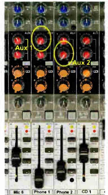
This setup allows a standard mixer to be used with phone couplers to provide a mix-minus to callers. Note Aux settings.
