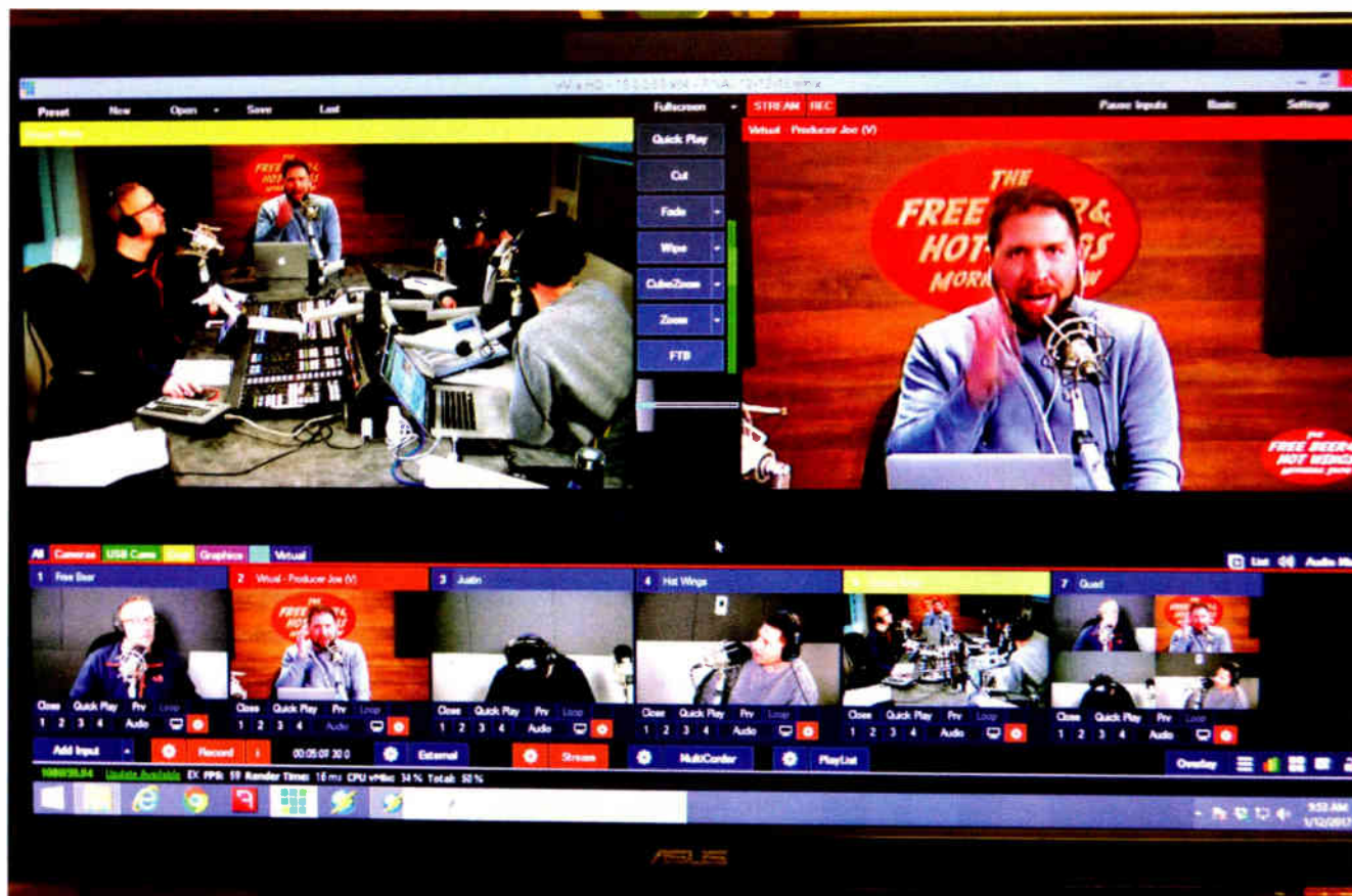
Four HD cameras feed a PC loaded with vMix switching software. Switching is automatic using a customized Arduino micro-controller that follows audio and is sourced from the show’s Wheatstone console.
