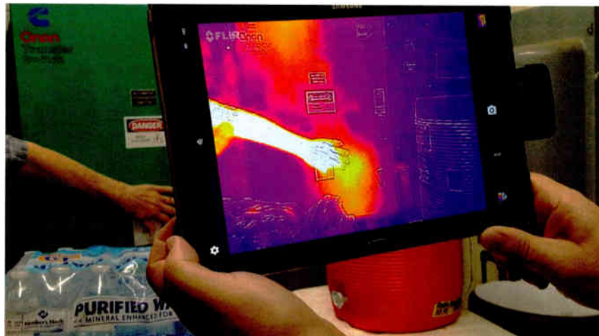
Fig. 4: ... and provides a visual display of heat-generating components.
