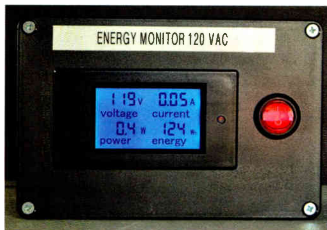
Fig. 1 (above): The meter measures voltage and current as well as power and energy.
