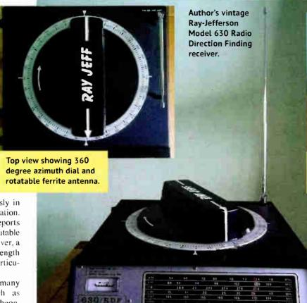
siasts or even AM DXers as auxiliary receivers because of their ability to null out unwanted AM signals on the broadcast band via the large rotatable ferrite
