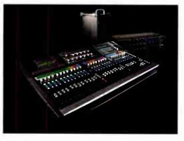
and "Number of Open Microphones" logic gate technology for a more flexible and sophisticated auto mix. A Best Mic Lock system detects crosstalk between various sources and limits open microphones.
