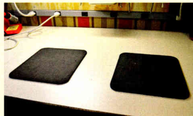
Fig. 4: Rubber side up; the equipment is cushioned yet can be moved easily.
