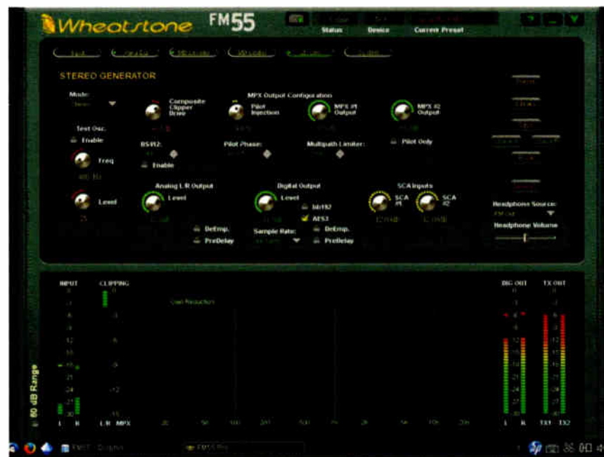
Fig. 3: The Multipath Limiter intelligently controls the L-R energy.
