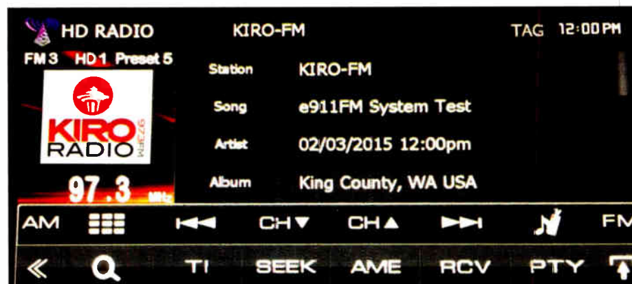
An HD Radio receiver displays an e911FM test message, broadcast by Seattle partner KIRO(FM).
