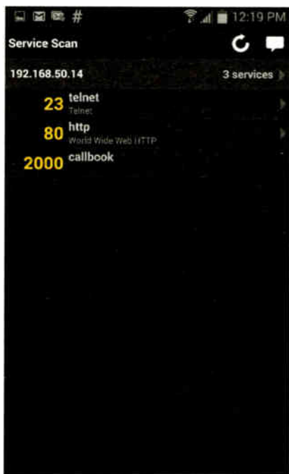
Fing can determine which Web services are available at a specific IP address.
