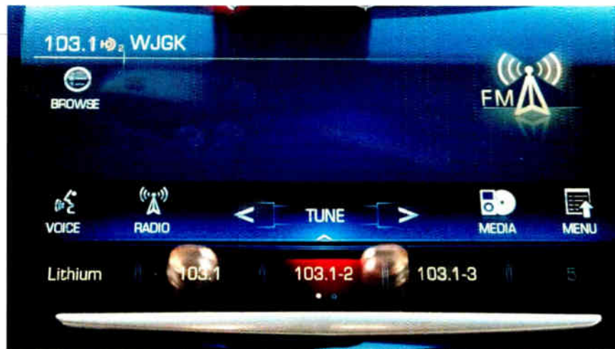
The HD1, HD2 and HD3 channels of WJGK(FM), Newburgh, N.Y., are displayed on the tuner in a Cadillac CTS.
