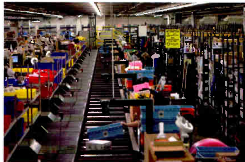
Workstations add and subtract items from the conveyor belt, which never stops. Bar code readers on green arms keep track of everything.
