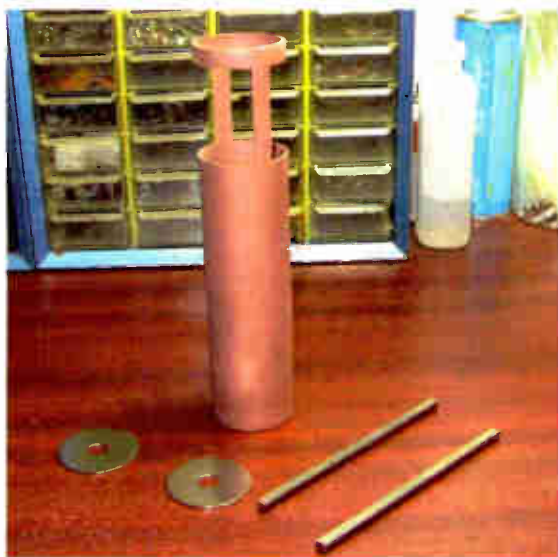
The mic body's main metal body materials are pictured.
