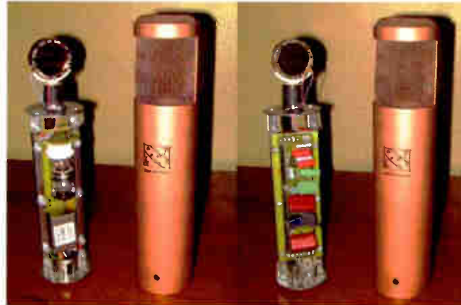
The completed G7 microphone with the tube/transducer side of the mic board PCB (left) and the back of the mic board PCB facing the viewer (right).
