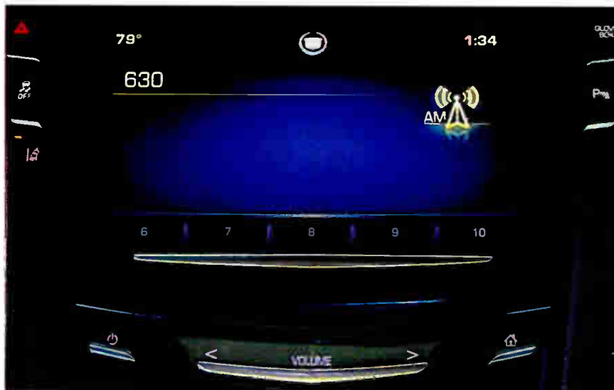
AM stands out as the only service in the car that currently can't display even analog artist and title data. AM becomes the 'blank screen' in the dash – the only 'unconnected' part of the connected car.
