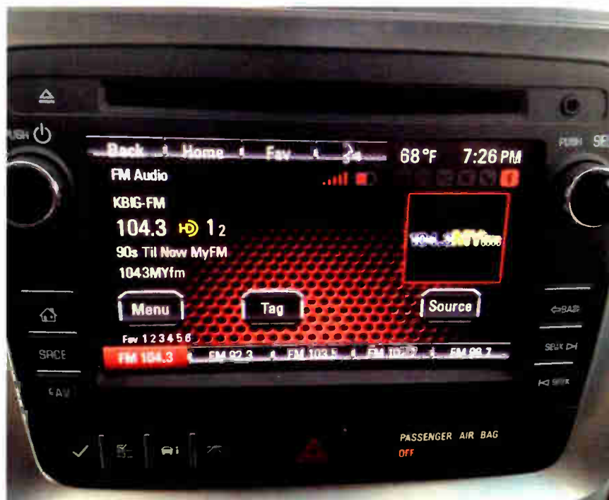
A typical implementation of HD Radio with Artist Experience in a 2013 GMC Acadia and Chevrolet Traverse. Both GM vehicles offer HD with AE standard. The author was listening to KBIG(FM) in Los Angeles when he took this photo.
