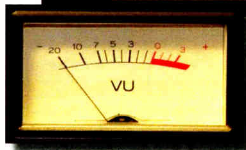
Audio level meters should adhere to the official VU standard for response to signals — but don't always, even if they are marked 'VU' on the face.
