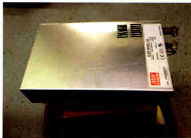
Fig. 1: The Mean Well replacement power supply for a BE FM1C1.
