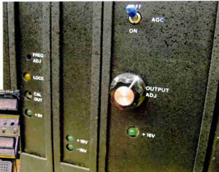
Power control knob as added to MX-15 exciter
