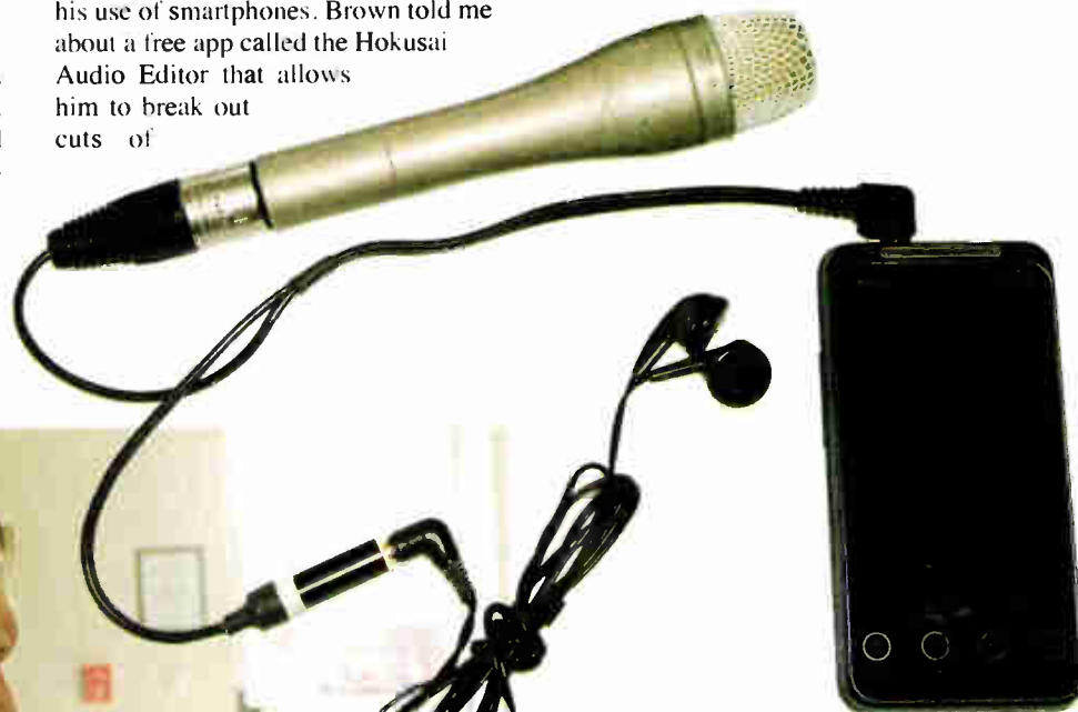
The Warrior's kV Connection configuration for using a dynamic mic with his Sprint EVO smartphone.
