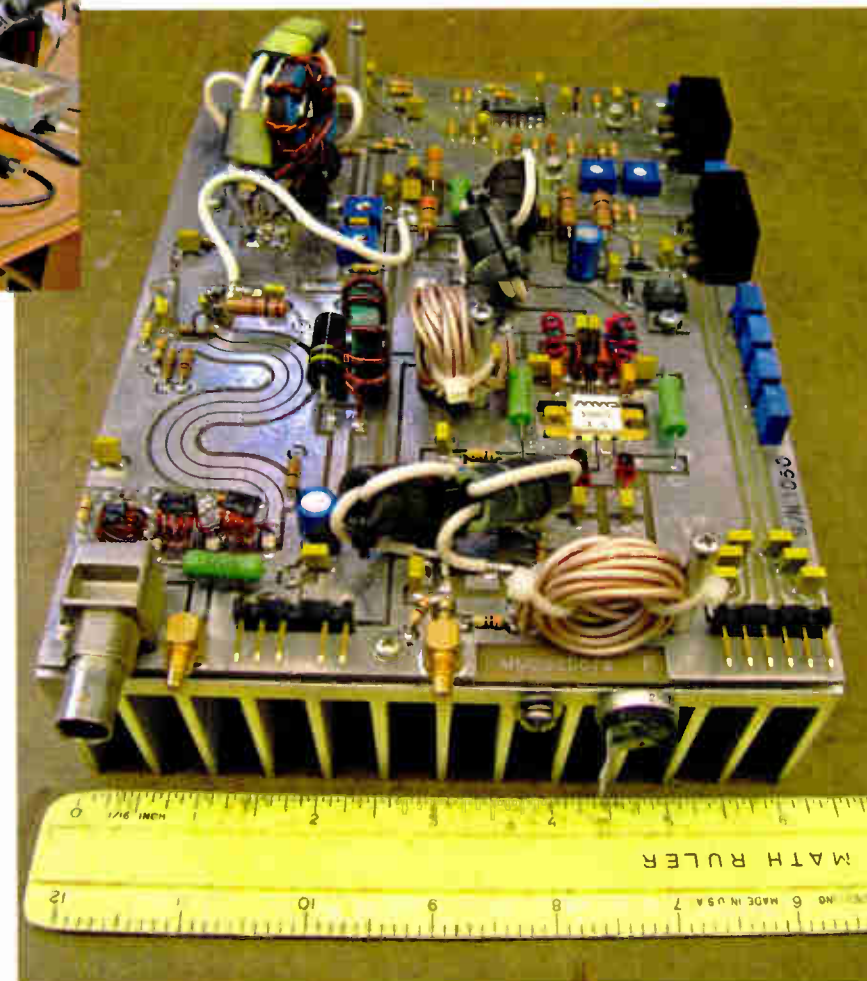
Original PA module in THE-1 exciter
