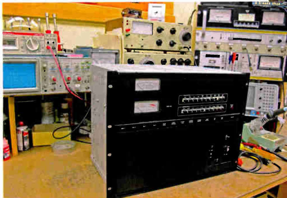
A Harris MX-15 exciter is shown on the testing bench.
