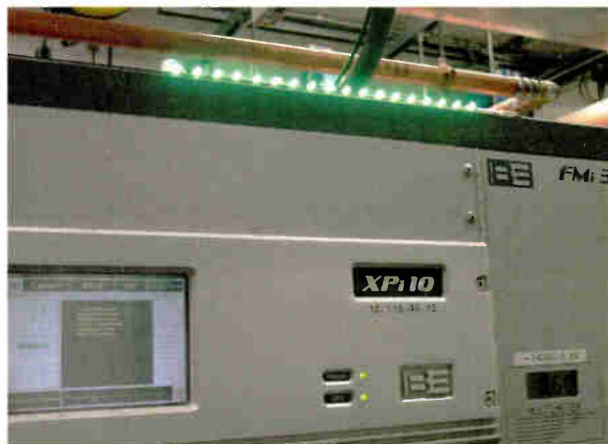
Fig. 3: LEDs, top, provide a quick visual indication to identify which transmitter is 'on the air.'
